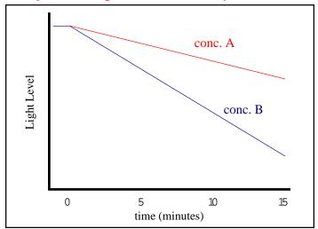
This Light Level-Time Response curve is typical of many heavy metal compounds. The decay rate of the light is essentially constant for an extended period of time, and depends on concentration. Response curves of this type indicate why multiple light readings (It) at 5, 15 and 30 minutes, are recommended.
