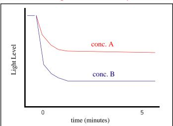
This Light Level-Time Response curve is typical of organic compounds. The light output drops somewhat more gradually than for phenol, then levels off.
